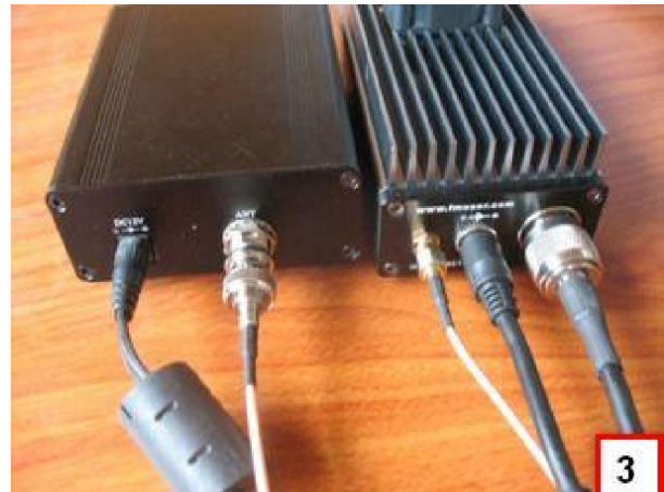
Picture3 Connect the amplifier and exciter respectively to power supply
