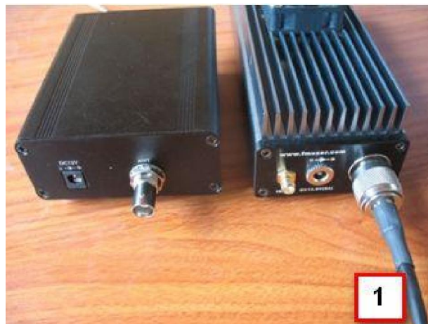
Picture 1 Connect the antenna and power amplifier
