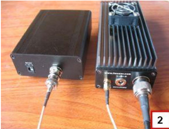
Picture 2 Connect the power amplifier to exciter with feeder line.
